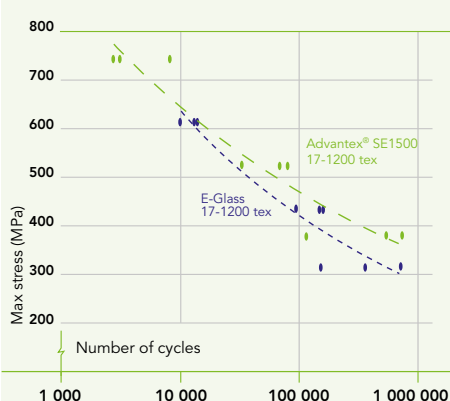
Tensile (R=0,1) fatigue of Epoxy UD laminates
