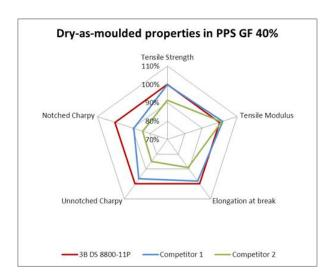
The optimized dispersion behaviour of DS 8800-11P allows its usage in a wide range of resin viscosities, also at very high glass fibre loading (>55%).
